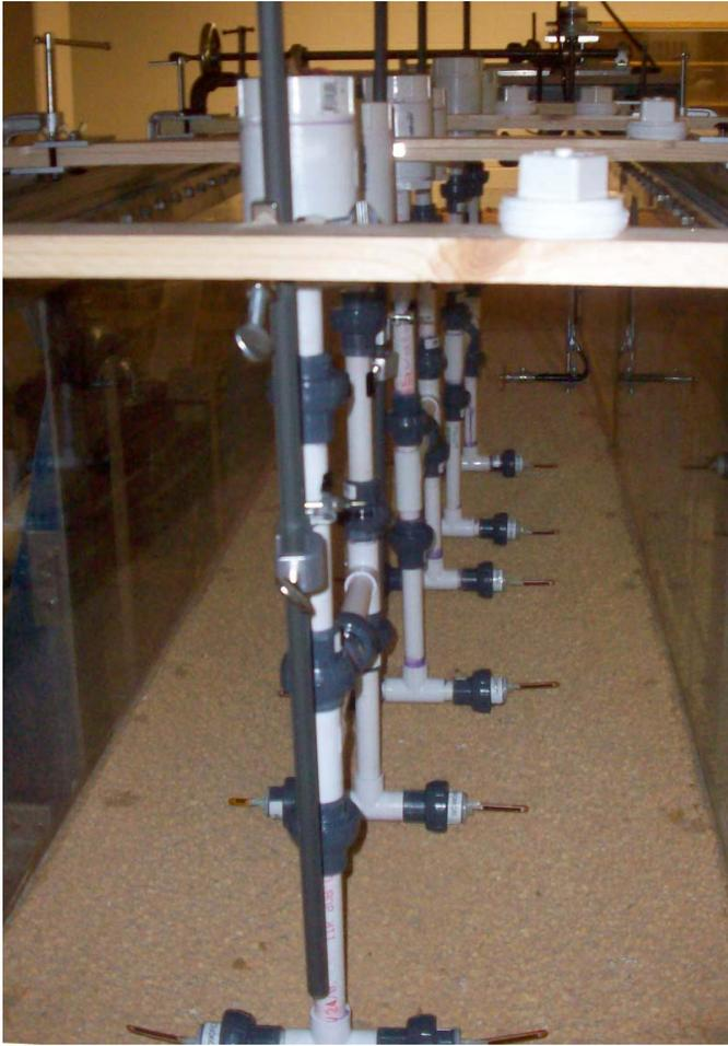
Fig. 3: Multiple sensors connected to wireless nodes before filling the flume. Sensors are oriented perpendicular to the flow at the base of the flume. The acoustic Doppler velocimeter appears at right after the row of sensors.
