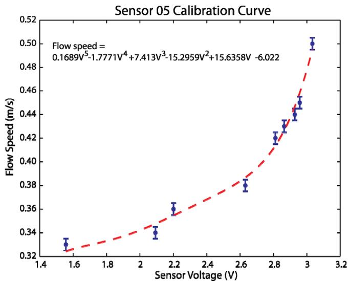
Fig. 5: Inverted calibration plot for a flexible sensor from flume tests. Calibration coefficients were obtained by a least-squares polynomial fit.
