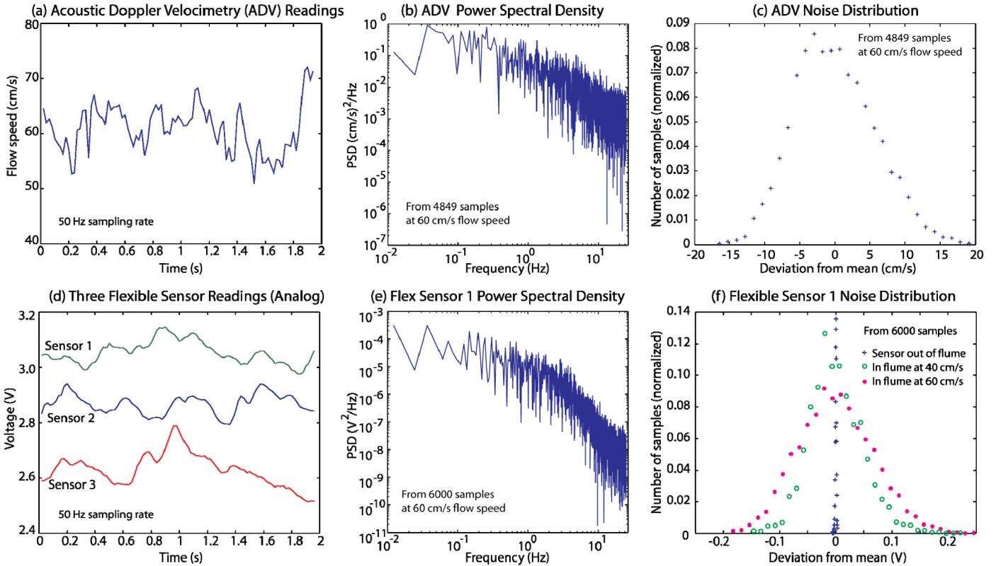
Fig. 2: Comparison of Acoustic Doppler Velocimeter and flexible flow sensors. (a) ADV time series, (b) ADV noise spectrum, (c) ADV fluctuation statistics, (d) time series for three flex sensors, (e) flex sensor noise spectrum, (f) flex sensor fluctuation statistics for two flow speeds and zero static deflection.
