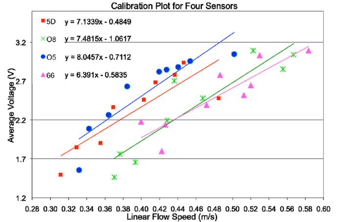
Fig. 4: Calibration plot for four different flexible sensors from flume tests. Calibration coefficients are obtained for each sensor by inverting the plots (speed-vs-voltage) and fitting the data.
