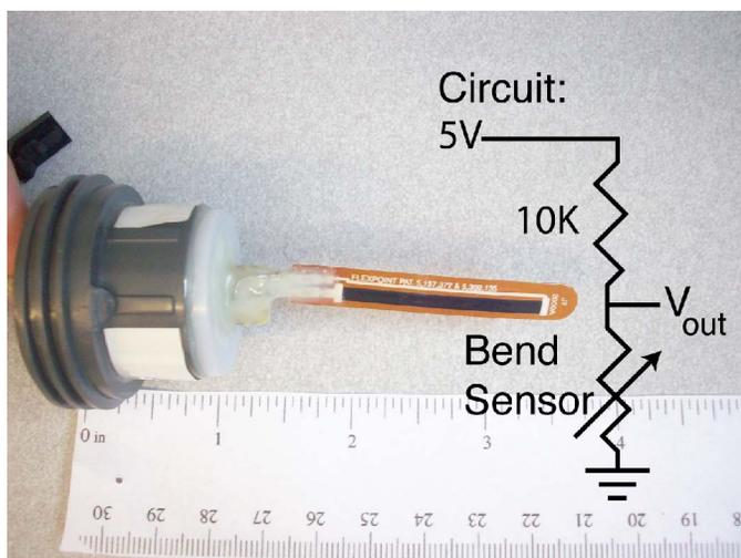
Fig. 1: A waterproofed Bend Sensor installed in a PVC pipe union and interfaced with a voltage divider and analog-to-digital converter chip.
