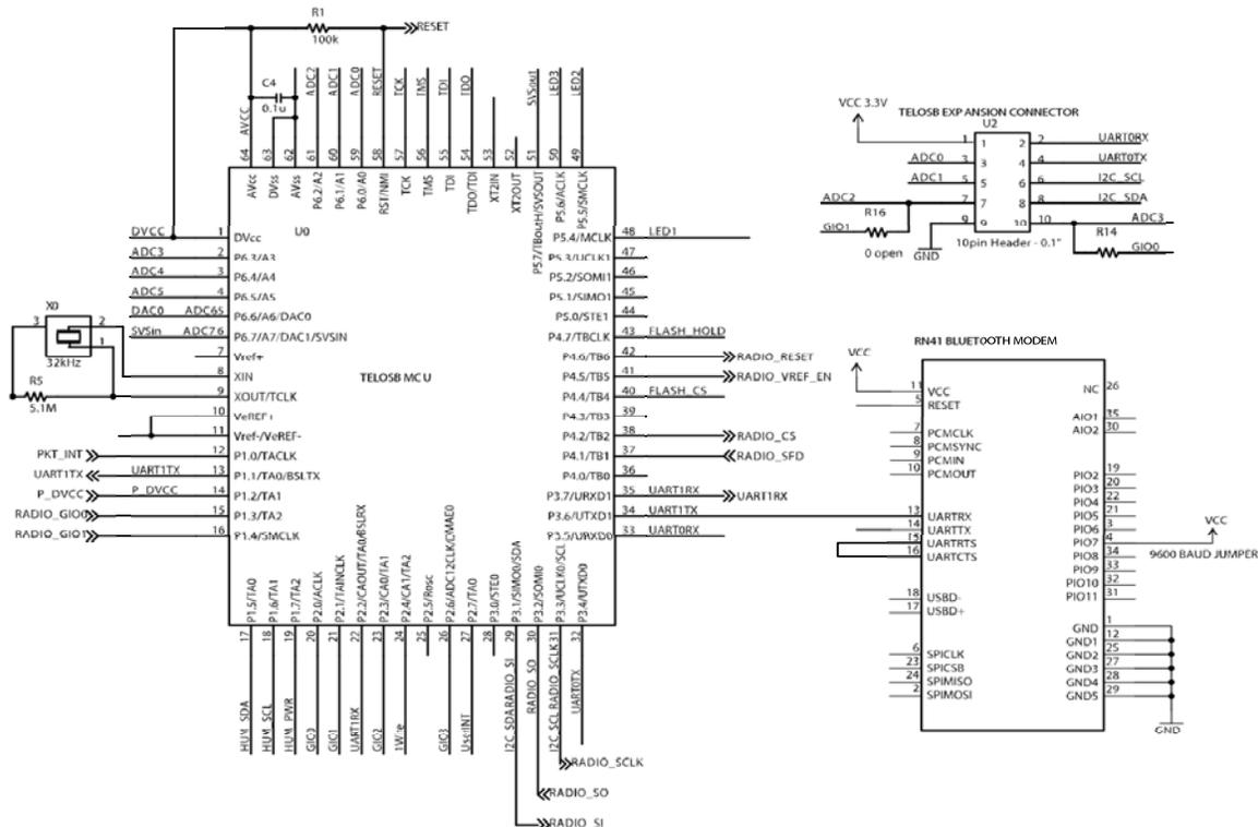
Figure 2: Wireless sensor network-Bluetooth gateway schematic.
