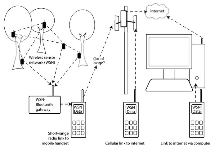
Figure 1: Wireless sensor network gateway for transmitting data to nearby mobile phones over a short-range radio link. Phones can upload stored data when in range of a cellular tower or internet-connected computer.
