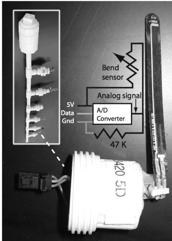
Figure 3: Inset: SALAMANDER with turbidity, pressure, temperature, and flow sensors (flow sensor shown enlarged with schematic of DS2450 A/D interface). Tmote Sky radio node and 4AA battery pack fit in top capsule. All sensors attach via ½-inch PVC pipe unions.
