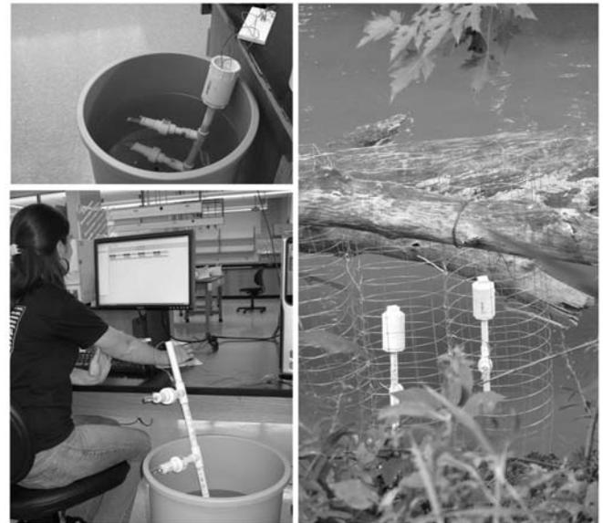
Figure 7: Clockwise from top left, leak checking a SALAMANDER in the laboratory; SALAMANDERS installed outdoors in protective cages with wireless nodes above water; determining individual serial numbers of attached sensors for programming a Tmote Sky wireless node.
