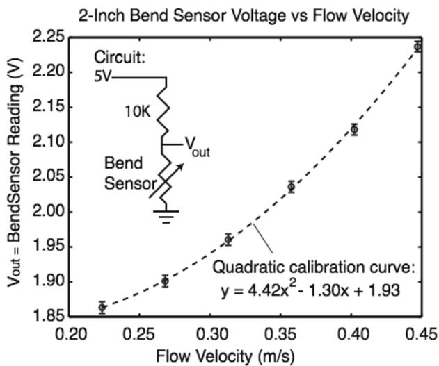
Figure 4: Measured voltage and resulting calibration curve for a water flow rate sensor based on the 2-inch long polyester-coated BendSensor. Flow velocity is determined from the voltage data by inverting the calibration curve, using the processor on the Tmote Sky or on the data collection computer.
