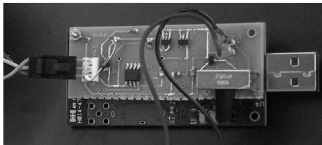
Figure 0: Power conversion board enables Tmote Sky module to interface with 1-Wire sensors. Three wires at left carry 5V, data, and ground to the sensor chain; wires at right go to a 6V battery pack.
