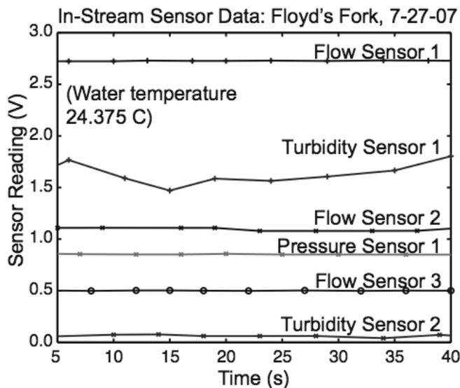
Figure 8: Time series of in-stream sensor data collected from four sensor types, at different depths, using two SALAMANDERS.
