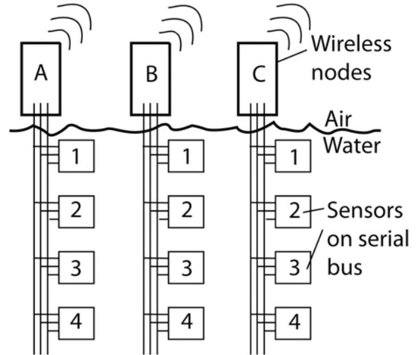
Figure 0: Set of wireless nodes with local wired networks of underwater sensors.
