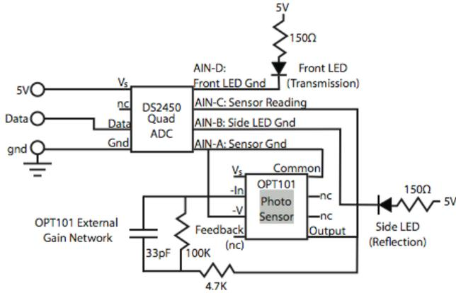
Figure 6: Circuit schematic for optical turbidity sensor based on OPT-101 photosensor and DS2450 analog-to-digital converter.
