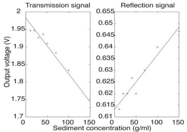
Figure 5: Low-power turbidity sensor uses red LEDs and an optical sensor to measure reflection and transmission through 1 to 3 cm of water. The sensor components are waterproofed by a vapor-deposited parylene coating.
