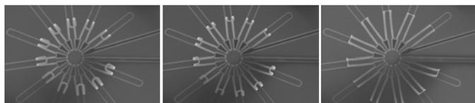
Fig. 2: Top view of a spherical microcage opening as temperature increases from 25C (left) to approximately 160C (right) by driving a current through the entire structure from contact pads to the right of each frame. Sphere diameter is 250 microns (leftmost image).
