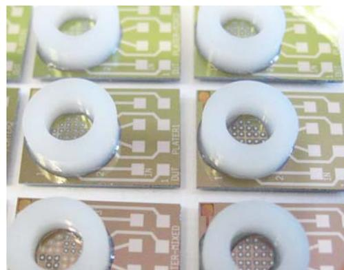
Fig. 3: Chips with sample wells and electrical contacts for collecting metal samples by electroplating. Sample well volume is 50 microliters.
